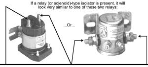
At the factory, the manufacturer has connected one of these large terminals to the positive terminal of your house battery bank. The other large terminal is connected to the positive terminal on your starting battery(s). You want to connect AMP-L-START's **HOUSE** [+] stud to the terminal that goes to the HOUSE batteries, and connect AMP-L-START's **STARTING** [+] stud to the terminal that goes to the STARTING battery(s).
