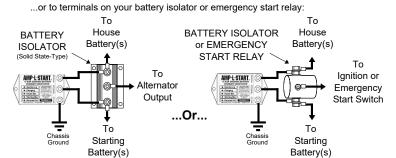
(NOTE: In dual starting battery applications, the connections can be made to either starting battery.)
