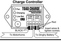
Attach a FEMALE connector to it, just like in STEP 5 above. Use another piece of surplus red and black wire to connect the Charge Controller to the dingy battery, using ring terminals to connect the wires to the dinghy battery cable clamp bolts or jump start terminals (Red wire to [+], Black wire to [-]).
