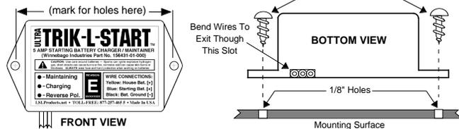
Determine how long the blue, yellow and black wires need to be in order to reach their intended connection locations, and cut off any excess wire. Strip approximately 1/4" (6 MM) of insulation off the ends of each of these wires, twisting any frayed strands back together again. Next, insert a ring terminal (supplied) into the end of each of these wires, and crimp the terminal tightly.
