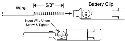
Next, use a pair of pliers to mash the battery clip's strain-relief tabs over the insulated portion of the wire, so that tugging on it doesn't separate the wire from the clip. Finally, slide the insulative boot down over the clip, so that only the clip's jaws are exposed. Do the same with the black wire, using the BLACK insulative boot instead.
