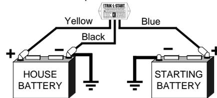
**TIP:** These connections can instead be made to terminals on the battery isolator, relay or selector switch — This helps avoid long wire runs and corroded clips. If additional wire is required, use 18 Gauge or thicker.
