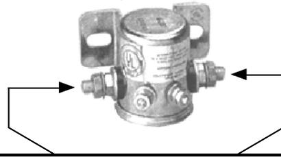
At the factory, the manufacturer has connected one of these large terminals to the positive terminal of your house battery bank. The other large terminal is connected to the positive terminal on your starting battery(s). You want to connect Trik-L-Start's YELLOW wire to the terminal that goes to the HOUSE batteries, and connect Trik-L-Start's BLUE wire to the terminal that goes to the STARTING battery(s).
